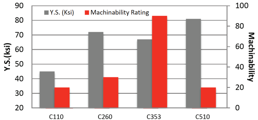
Figure 1: Comparison of Yield Strength and Machinability performance of select Hard temper copper based materials.
